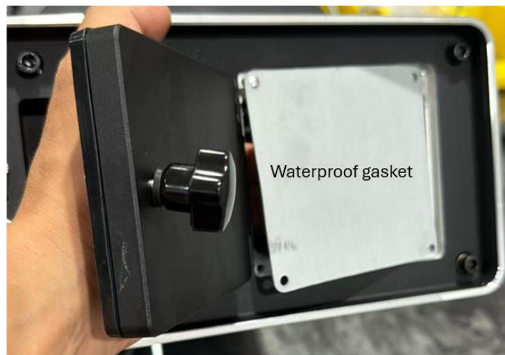
Figure 9 remove waterproof gasket of the electrical access port
