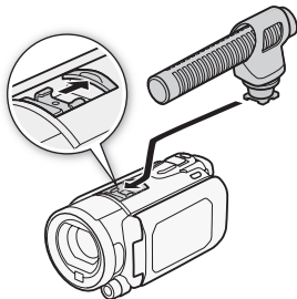
Example: Attaching an optional DM-100 Directional Stereo Microphone.
