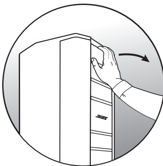
Pulling the array out
