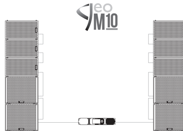
NXAMP4X2MK2 powering 3 X GEO M10 and 2 X MSUB15 per side
