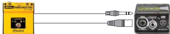
The JR1 uses either 1/4" or locking XLR cable to connect to the Relay Xo.
