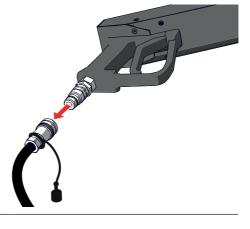
**6** Disconnect the  $CO_2$  hose from the  $CO_2$  Bottle to Hose Connector on the  $CO_2$  cylinder.
