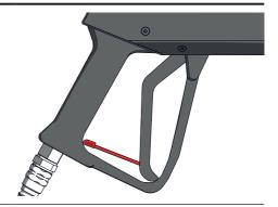
5 Disconnect the  $CO_2$  hose from the  $CO_2$  quick connector on the gun.
