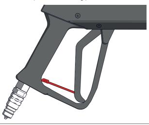
2 Connect the CO<sub>2</sub> hose to the CO<sub>2</sub> quick connector.
