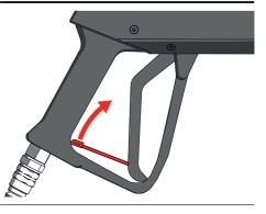
3 Squeeze the handle to release the remaining pressure.
