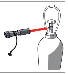
4 Connect the  $CO_2$  hose to the  $CO_2$  Bottle to Hose Connector on the  $CO_2$  cylinder.
