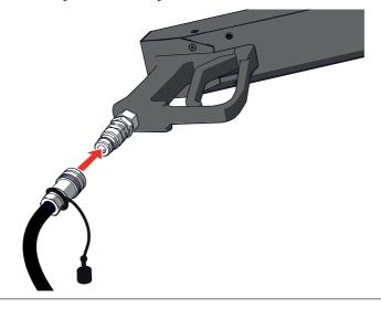
3 Connect the CO<sub>2</sub> Bottle to Hose Connector to a CO<sub>2</sub> cylinder.
