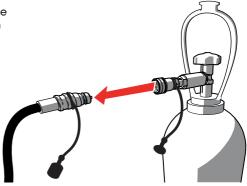
7 Remove the CO<sub>2</sub> Bottle to Hose Connector from the cylinder.
