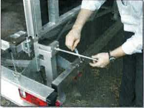
Steady legs for easy levelling of the stage floor
